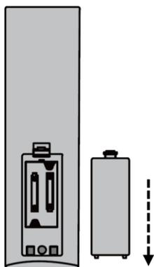
Open the battery compartment on the back of the remote control by sliding the cover off the remote control in the direction of the arrow.
