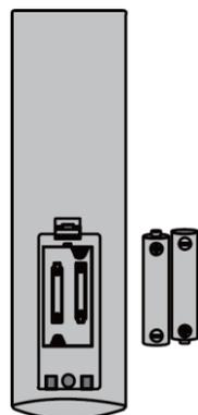
Remove the batteries already inserted and insert the new batteries into the remote control. When inserting the batteries, pay attention to the polarity (+/-) in the battery compartment.
